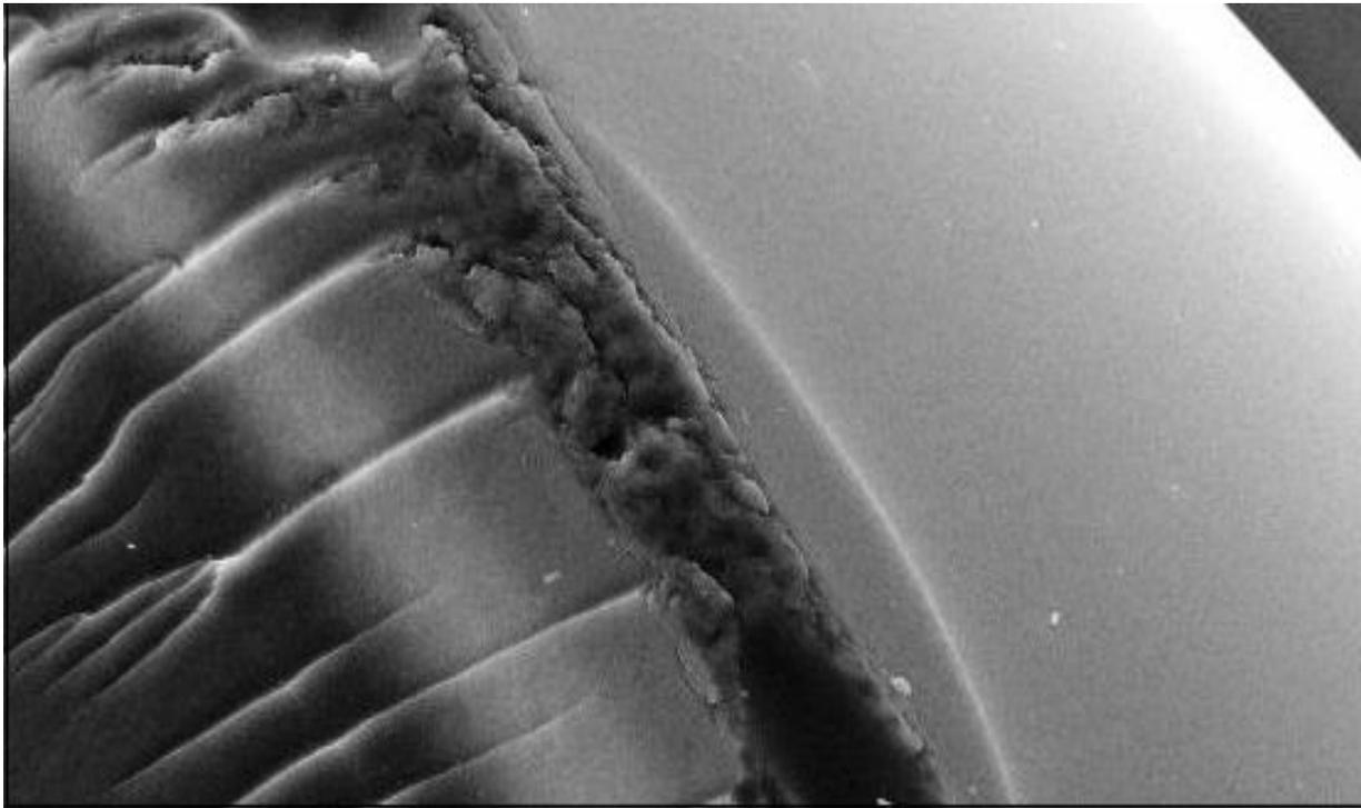
Figure 4: 1500X magnification SEM photo of a gel resin showing surface characteristics. Left side of SEM shows stress fracture of weaker gellular structure. Right side of SEM shows no discernable transport pores to access internal surface area required for adsorption reactions to occur.
