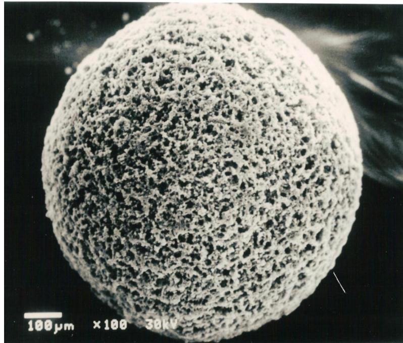
Figure 1: Scanning Electron Microscope photo of Tulsion T-45 BD Macro magnified 100X.
