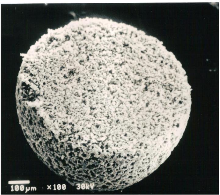
Figure 3: 100X magnification showing cross-sectional scanning electron microphotograph of Tulsion T-45 BD Macro
