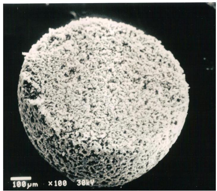
Figure 3: 100X magnification showing cross-sectional scanning electron microphotograph of Tulsion T-45 BD Macro
